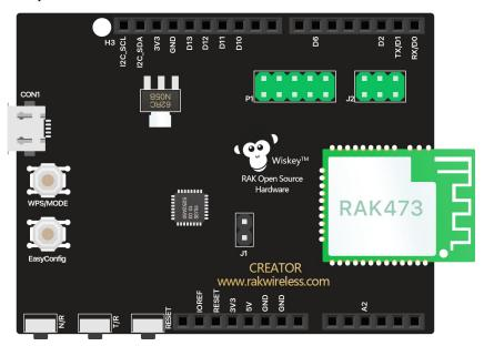
CREATOR pro and Arduino Uno have similar size, and the pins on CREATOR pro are compatible with Arduino Uno.
