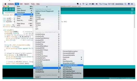
② Modify the tag part of the SSID and password, so that CREATOR pro connected to the router.
